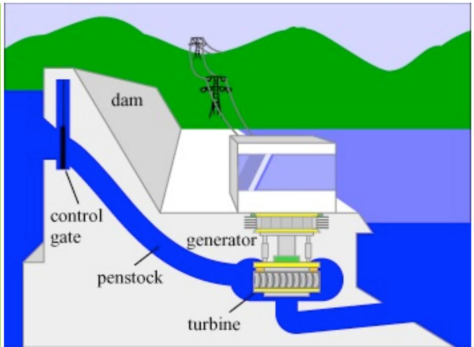
In a hydroelectric power plant, water from the upper reservoir is controlled to flow through the dam to turn the turbine generator.
