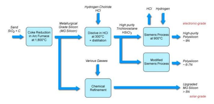
There are three main categories of manufacturing processes, resulting in different purity levels:
