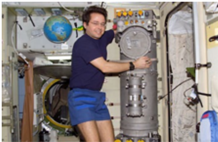
Astronaut Daniel W. Bursch, Expedition Four flight engineer, works on the Elektron Oxygen Generator in the Zvezda Service Module on the International Space Station (ISS).
